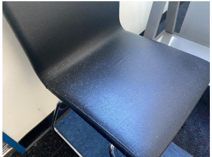
Photo #8: Bldg C, Classroom 14 - visible smoke related particulate on contents located directly adjacent to exterior entry points (<5 ft.)
